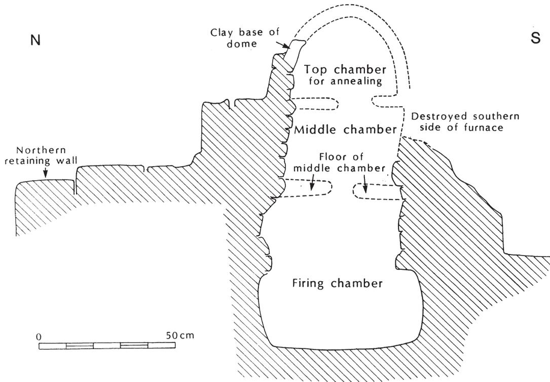
Fig. 2 — A north-south cross section through an 8<sup>th</sup>-9<sup>th</sup> century bee-hive shaped glass furnace found at Tell Zujaj, al-Raqqa, one of three glass production sites excavated.
